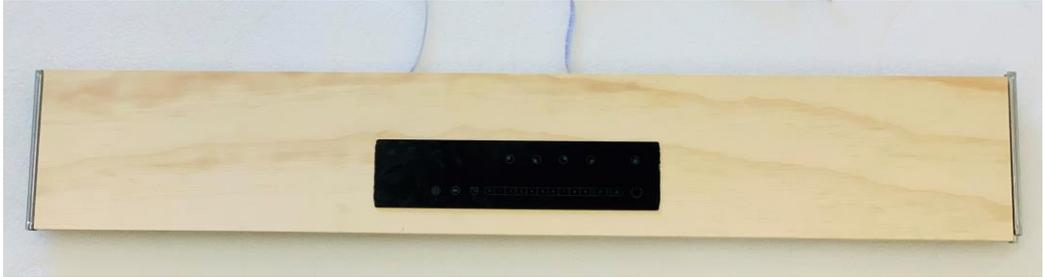
Step 4 is to feed the wires thru the wholes on both side and then connect controller. Once connected, drop the controller in so it sits flush to within the frame, and power it on.
